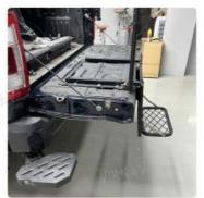
Special locking device, after use, the ladder can be securely locked onto the tailgate
