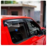
Window sunshades can block rainwater while allowing fresh air to circulate, allowing for gentle opening of windows even during rain.
